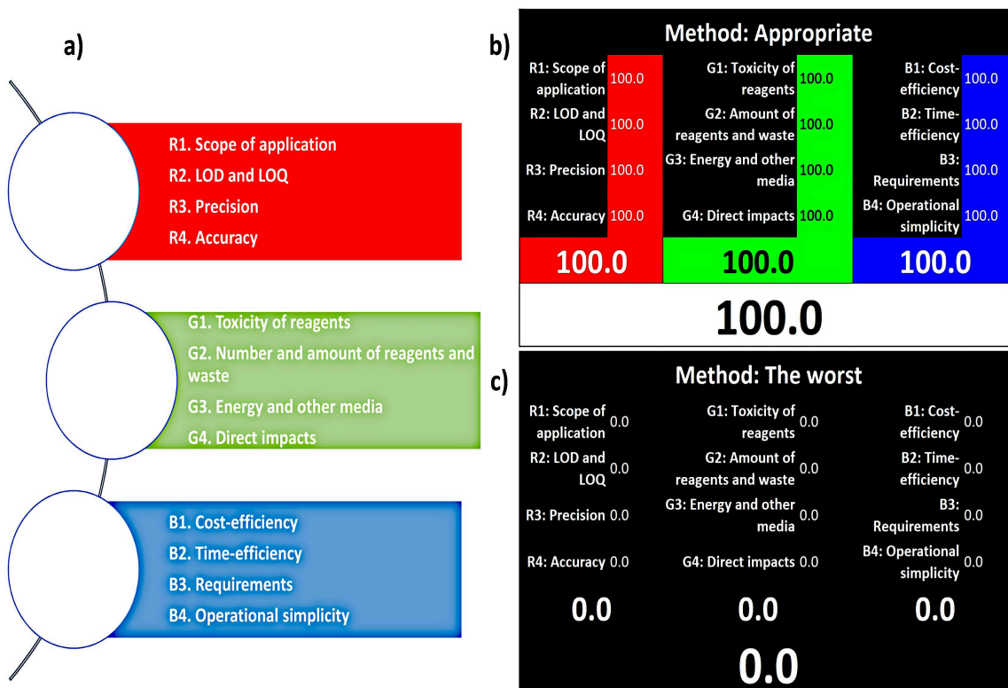
Figure 7. a) The 12 principles of white analytical chemistry (WAC); The result of the RGB 12 assessment for: b) a method that agrees with all WAC principles; c) a method that does not agree with any of the WAC principles.
