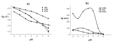
**Fig. 2** The influence of the pH on CV peak a) potential; b) current response for  $2 \times 10^{-5}$  M of CTRX (●),CFZ (■) and CFXA (▲), in BR buffer pH 2-8; v = 40 mV/s.
