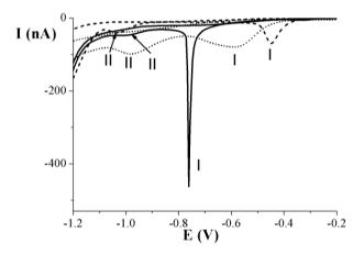
Fig. 1 Representative cyclic voltammograms of 2×10<sup>-5</sup> M CTRX (—), CFZ (····) and CFXA (----), at pH 4;  $v = 40 \text{ mVs}^{-1}$ .
