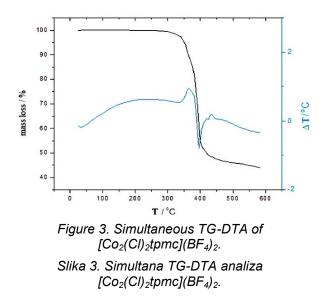
This complex is stable up to 310°C. The complex decomposes exothermally at 365°C. The curve of this complex reveals that decomposes at one step showing endothermic peak at 395°C and two exothermic peaks at 365 and 435 °C in DTA.
