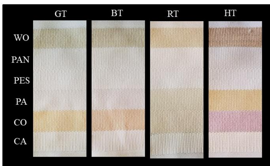
Fig 3. The appearance of the dyed multifiber fabric using different tea aqueous extracts
