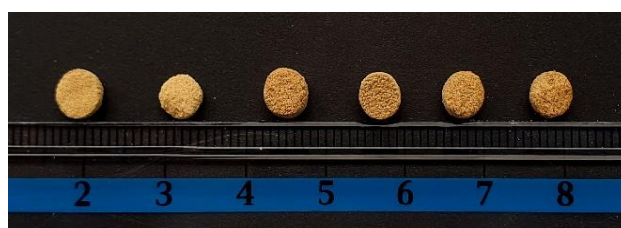
Figure 2. Photographs of the selected SLS-printed tablets with irbesartan. Tablets were printed with different laser speeds. From left to right: 100.00 mm/s, 120.00 mm/s, 140.00 mm/s, 160.00 mm/s, 180.00 mm/s, and 220.00 mm/s.
