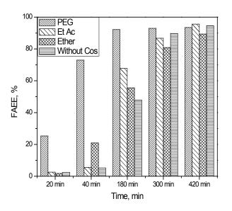
**Figure 4.** The FAEE yield obtained by catalytic reaction with CaO as catalyst without cosolvents and in catalytic reactions with CaO as a catalyst with the following cosolvents: propylene glycol , ethyl acetate and diethyl ether . Reaction conditions: catalyst concentration, based on the oil weight 1.3736 mol·dm<sup>-3</sup>; temperature 70 °C; and ethanol-to-oil molar ratio 12:1.
