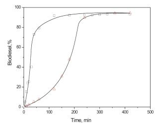
**Figure 1.** The variations of the FAEE yield with the progress of sunflower oils ethanolysis catalysed by CaO (20%, based on the oil weight): no cosolvent -  $\circ$ ; with propylene glycol (PEG) as cosolvent -  $\Box$ . Reaction conditions: catalyst concentration, based on the oil weight 1.3736 mol·dm-3; temperature 70 °C; and ethanol-to-oil molar ratio 12:1.
